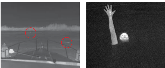
The Mariner can resolve people and objects in the water at night. The man overboard and the log in the river are clearly visible from the craft.
